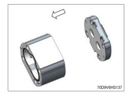
(16) Reassemble thrust plates and gears.
