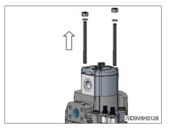
(8) Remove the screws and washers from gear pump section.
