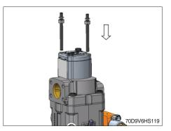
(23) Reassemble the nut, washers and stud bolt. • Tightening torque : 4.6 kgf·m (33.3 lbf·ft)
