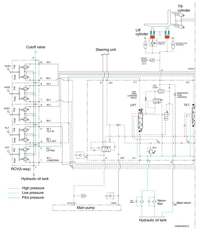
When the lift control lever is pulled back, the lift spool in the first block is moves to lift position. The oil from the main pump flows into the lift spool of main control valve through the priority valve. Then goes to the large chamber of lift cylinder by pushing the load check valve of the spool and lift lock valve. The oil from the small chamber of lift cylinder returns to hydraulic oil tank at the same time. When this happens, the forks go up.
