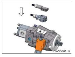
(29) Tighten the bolts with a torque wrench. • Tightening torque : 1.5 kgf·m (10.9 lbf·ft)
