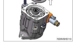
(18) Use grease in order to attach valve plate to the cover, following the pin.
