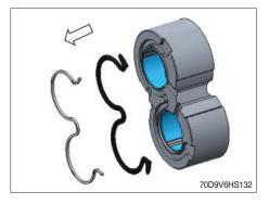
(11) Insert new seal and anti-extrusion seal.
