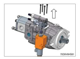
(2) Remove the pressure and the flow compensators.
