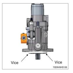
(6) Remove the nut from stud bolt from gear pump section.
