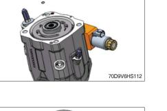
(17) Remove the valve plate.
