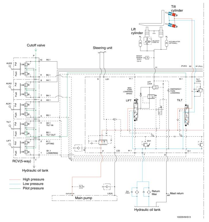
When the tilt control lever is pushed forward, the tilt spool in the second block is moved to tilt forward position.
