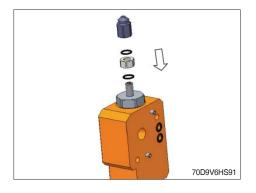
(12) Remove the O-ring seals on the compensator plane.
