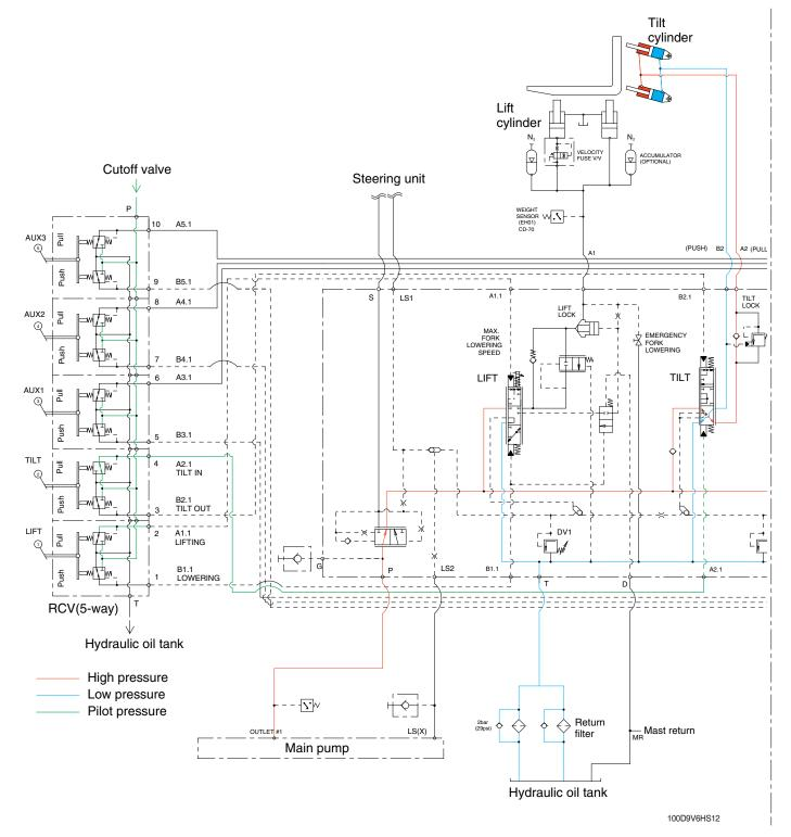
When the tilt control lever is pulled back, the tilt spool in the second block is moved to tilt backward position.
