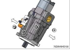
(7) Remove the screws and washers from gear pump section.
