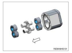
(10) Remove seal and anti-extrusion seal.
