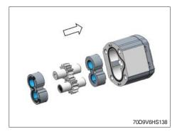
(17) Reassemble the gear pump section.
