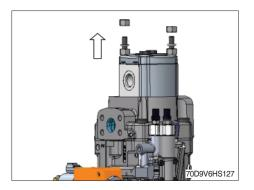
(7) Remove the nut, washers and stud bolt from gear pump section.
