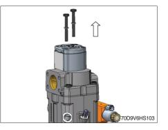
(8) Remove the gear pump section.
