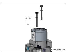
(8) Remove the gear pump section.
