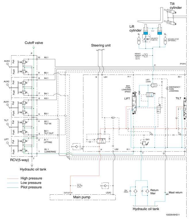
When the lift control is pushed forward, the lilt spool in the first block is moved to lower position. The work port and the small chamber and the large chamber are connected to the return passage, so the forks will be lowered due to its own weight.
