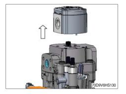
(9) Remove thrust plates and gears from the housing.
