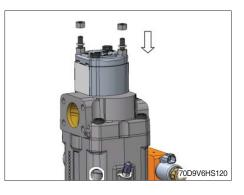
(25) Remove the O-ring from the drain plugs.
