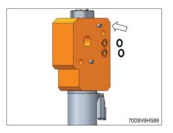
(10) Remove plug, nut and the O-ring seals.
