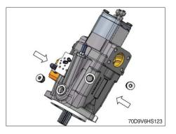
(28) Reassemble the flow and the pressure regulators.
